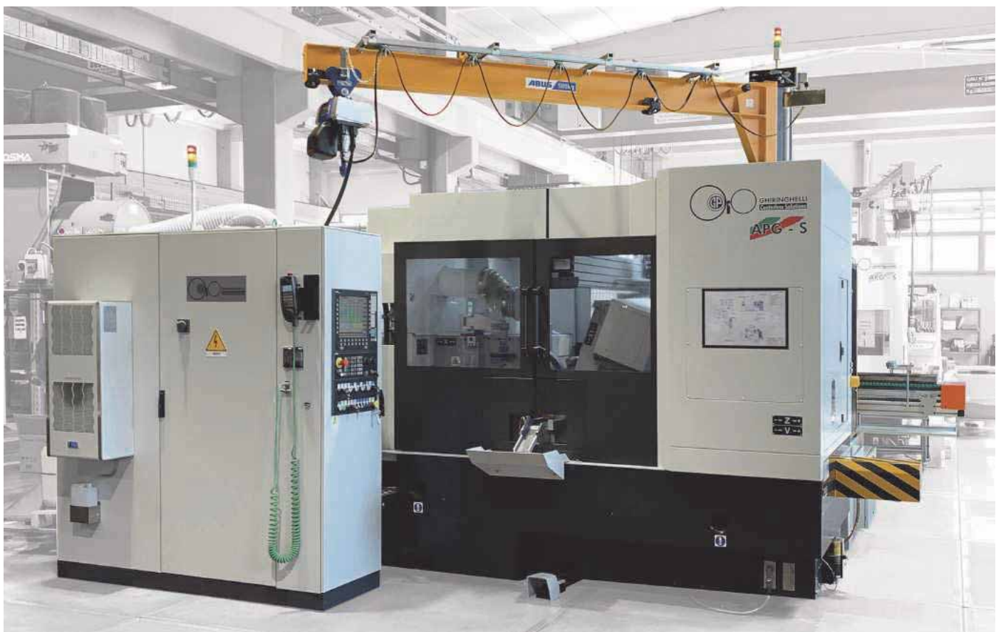
The new Ghiringhelli APG is designed for the optimal use of the centerless grinding process at high cutting speed up to 120 m/s
