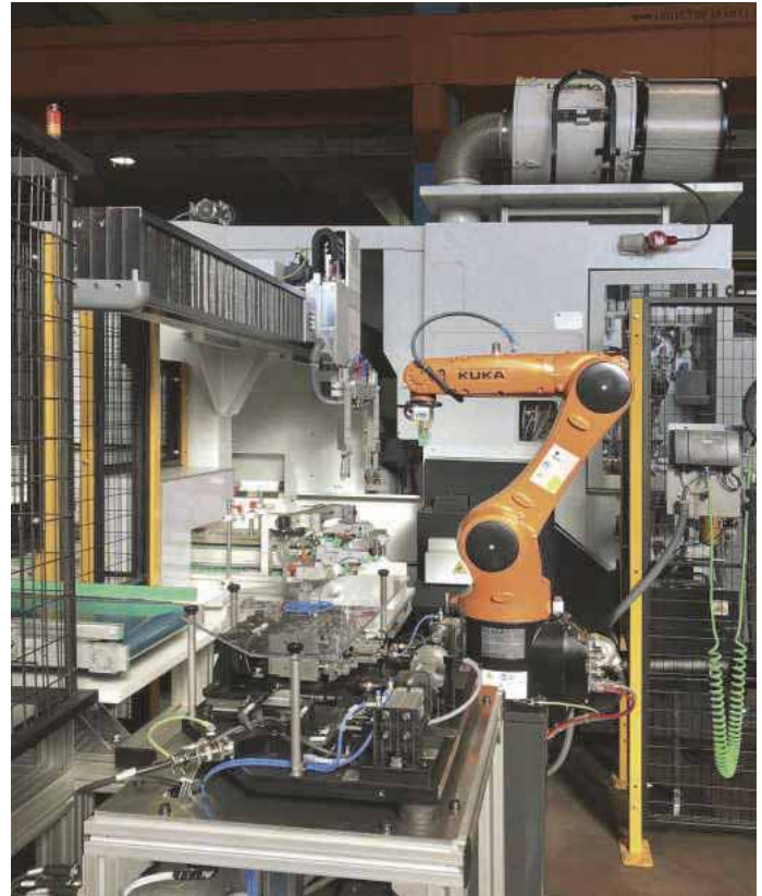
The Ghiringhelli centerless grinding machines can be equipped with automatic piece feeding systems and with post-process measuring systems used for machine correction
