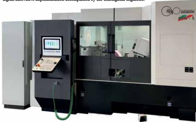
The brand new Siemens Sinumerik ONE control is the first CNC "digital native" which allows the creation of a digital twin (DT).
